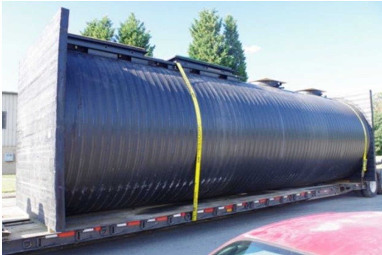
10,000 Gallon per Day Industrial Membrane Bioreactor Waste Water Treatment Plant designed by Daniel M. Early, PE, using long-lived Structural Reinforced ThermoPlastic (SRTP)
