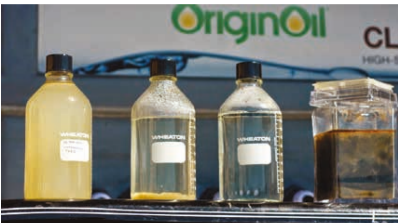
Figure 3. From left: feed water, separated water, final stage clean water and recoverable oil product.
